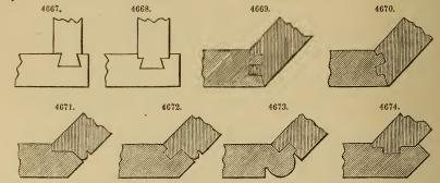
Figs. 4669 to 4674 show the same kind of joints as have been described, applied to the framing together of boards meeting in an obtuse angle.
